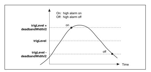
Figure 2-1. High Alarm Deadband
